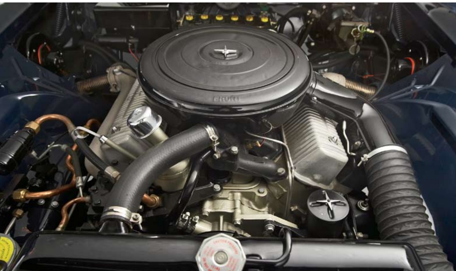
The Continental 300hp 368-cu.in. V-8 and driveline remained unchanged when Hess and Eisenhardt removed the Mark II's damaged roof
